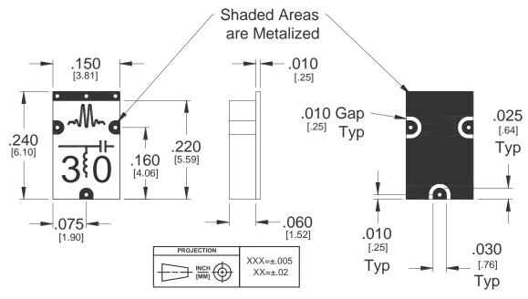
Substrate material is 10-mil thick Rogers 5880 or Taconic TLY-5, ½ Oz Electrodeposited Cu. I/O Pads & Ground Plane Finish is Gold Flash, 5 to 10 μ-inches, over Solderable Electroless Nickel, 100-200 μ-inches, over Cu. See <a href="http://www.markimicrowave.com/menus/appnotes/an-btsm-pcb.pdf">http://www.markimicrowave.com/menus/appnotes/an-btsm-pcb.pdf</a> for suggested PCB layout.
