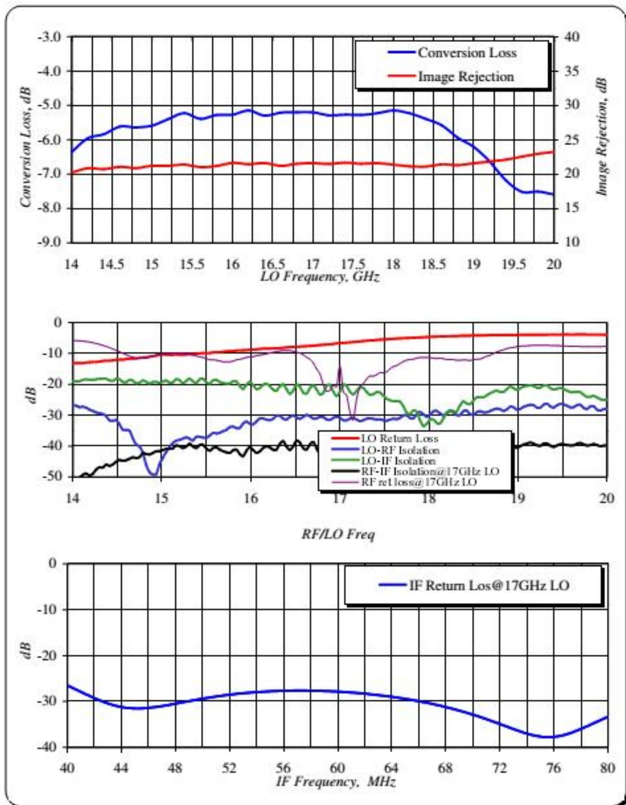
Typical measured data @ 25C with LO power = -3 dBm
