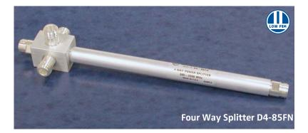
Microlab Model Dx-85FN series of 2, 3, 4, 5 and 6 way Power Splitters has been designed to evenly split high power cellular signals with minimal reflections or loss. All joints are moisture sealed to meet the IP67 rating. The design allows simple attachment to wall using the supplied bracket and clip.
