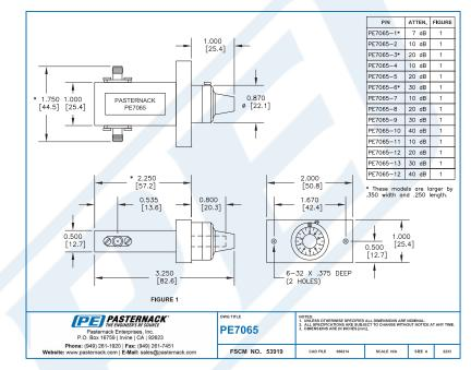
0 to 7 dB Rotary Continuously Variable Attenuator, SMA Female To SMA Female Rated To 5 Watts From 1000 MHz To 2 GHz from Pasternack Enterprises has same day shipment for domestic and International orders. Our RF, microwave and millimeter wave products maintain a 99% availability and are part of the broadest selection in the industry.
