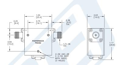
50 Ohm SMA Isolator Operating From 4 GHz to 8 GHz And 10 Watts With 18 dB Isolation from Pasternack Enterprises has same day shipment for domestic and International orders. Our RF, microwave and fiber optic products maintain a 99% availability and are part of the broadest selection in the industry.
