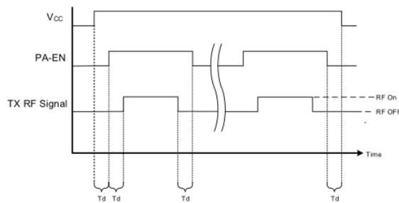
Note: Observe the timing sequence shown in the diagram above and described below. DC and RF signal levels per data sheet specification
