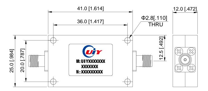
Unit: mm/ inch, General part tolerance is ±0.2mm unless otherwise stated.
