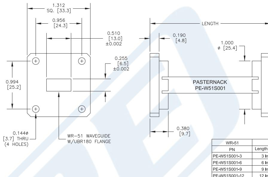
WR-51 Instrumentation Grade Straight Waveguide Section 12 Inch Length with R180 Flange Operating from 15 GHz to 22 GHz from Pasternack Enterprises has same day shipment for domestic and International orders. Our RF, microwave and millimeter wave products maintain a 99% availability and are part of the broadest selection in the industry.
