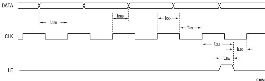
**Figure 3. SKY73103-11 Serial Data Input Timing Diagram (MSB First)**
