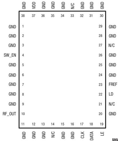
**Figure 1. SKY73103-11 Pinout– 38-Pin MCM Package (Top View)**
