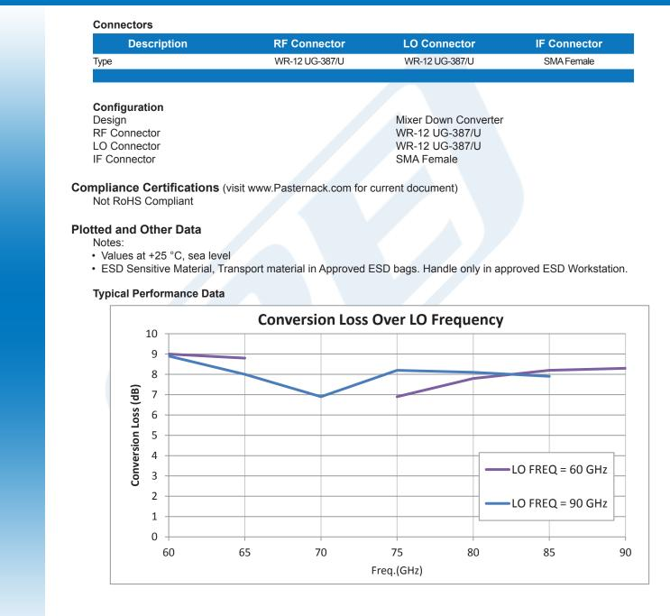
Click the following link (or enter part number in "SEARCH" on website) to obtain additional part information including price, inventory and certifications: Waveguide Mixer Down Converter WR-12 From 60 GHz to 90 GHz, IF From DC to 18 GHz And LO Power of +13 dBm, UG-387/U Flange, E Band PE12D1001
