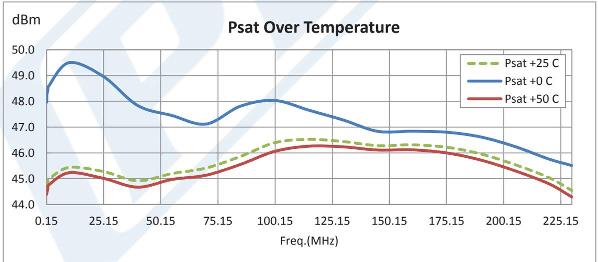
Click the following link (or enter part number in "SEARCH" on website) to obtain additional part information including price, inventory and certifications: [43 dB Gain, 25 Watt Psat, 0.15 MHz to 230 MHz, High Power High Gain Amplifier, 48 dBm IP3, SMA PE15A5028](#)
