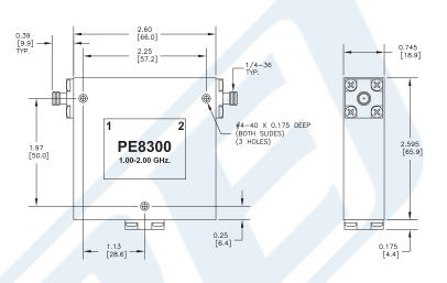
50 Ohm SMA Isolator Operating From 1 GHz to 2 GHz And 10 Watts With 18 dB Isolation from Pasternack Enterprises has same day shipment for domestic and International orders. Our RF, microwave and fiber optic products maintain a 99% availability and are part of the broadest selection in the industry.
