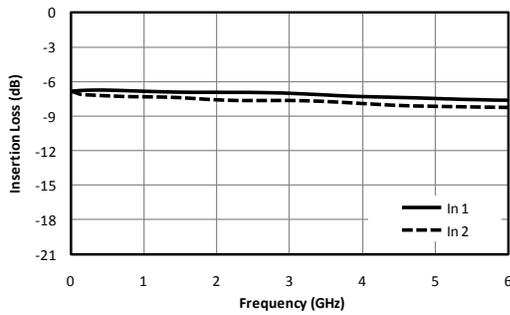
Fig. 3. Input port to common port insertion loss.
