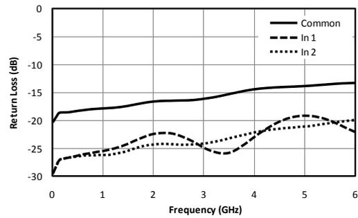
Fig. 4. Return loss for input and common ports.
