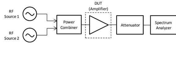
Fig. 2. Amplifier IP3 measurement
