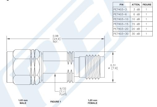
30 dB Fixed Attenuator, 1.85mm Male To 1.85mm Female Passivated Stainless Steel Body Rated To 1 Watt Up To 65 GHz from Pasternack Enterprises has same day shipment for domestic and International orders. Our RF, microwave and millimeter wave products maintain a 99% availability and are part of the broadest selection in the industry.
