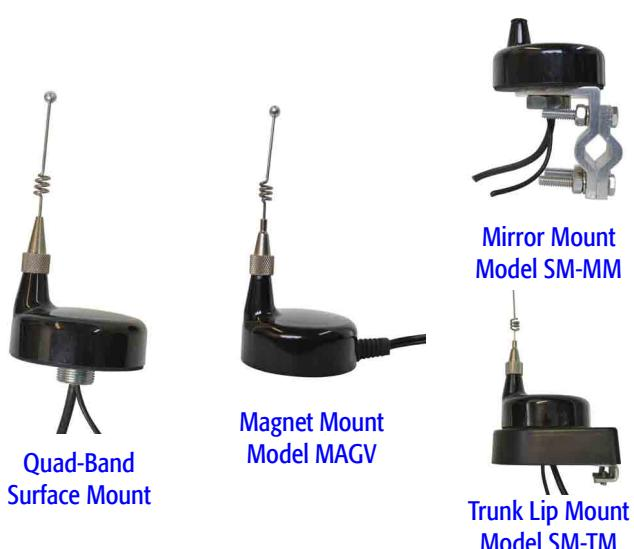
This antenna provides a high level of integration for Fleet Management & AVL tracking applications in a permanent thru-hole mount. The Quad-band Surface mount provides operation on all Cellular and PCS bands worldwide along with GPS. The GPS antenna has an active amplifier for maximum satellite reception.
