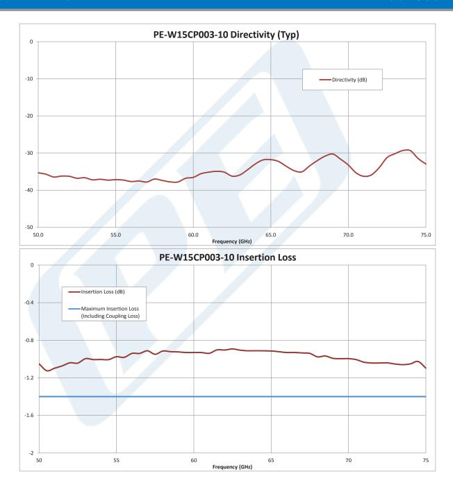
Click the following link (or enter part number in "SEARCH" on website) to obtain additional part information including price, inventory and certifications: WR-15 10 dB Directional Waveguide Coupler With UG-385/U Flange and E-Plane Coupled Port From 50 GHz to 75 GHz V Band PE-W15CP003-10
