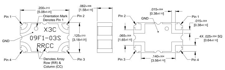
Dimensions are in Inches [Millimeters] X3C09F1-03S Mechanical Outline
