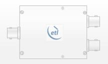
10dB L-band directional coupler with DC and 10MHz pass between input and transmit ports. The coupled port is DC blocked.
