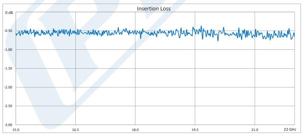
Click the following link (or enter part number in "SEARCH" on website) to obtain additional part information including price, inventory and certifications: WR-51 Flexible Straight Waveguide Section 24 Inch Length with Square Cover Flange Operating from 15 GHz to 22 GHz PE-W51SF005-24
