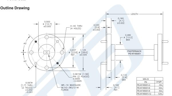
WR-19 Instrumentation Grade Straight Waveguide Section 3 Inch Length with UG383/U-Mod Flange Operating from 40 GHz to 60 GHz from Pasternack Enterprises has same day shipment for domestic and International orders. Our RF, microwave and millimeter wave products maintain a 99% availability and are part of the broadest selection in the industry.
