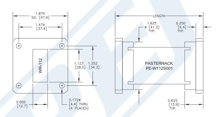
WR-112 Commercial Grade Straight Waveguide Section 6 Inch Length with UG-51/U Flange Operating from 7.05 GHz to 10 GHz from Pasternack Enterprises has same day shipment for domestic and International orders. Our RF, microwave and millimeter wave products maintain a 99% availability and are part of the broadest selection in the industry.
