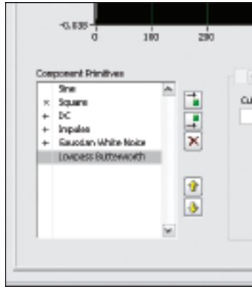
Figure 6: Over 20 different waveform primitives can be combined to create more complex waveforms.
