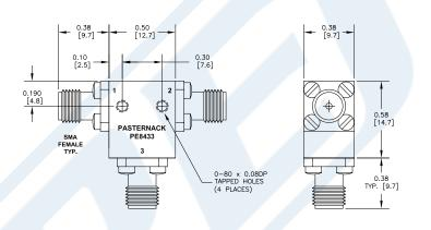
50 Ohm SMA Circulator Operating From 6 GHz to 18 GHz And 10 Watts With 14 dB Isolation from Pasternack Enterprises has same day shipment for domestic and International orders. Our RF, microwave and millimeter wave products maintain a 99% availability and are part of the broadest selection in the industry.
