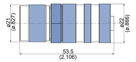
NOTE: (1) Snap on N plug with locking mechanism
