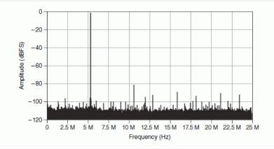
NI 5751 Characteristic Noise Density, Spectrum-64 k Samples
