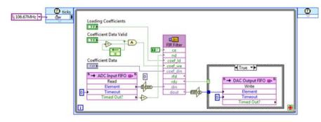
Figure 6. LabVIEW FPGA Code for an Inline Filter
