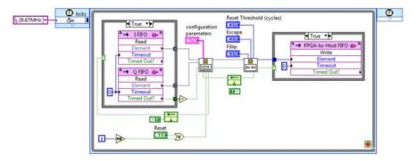
Figure 4. LabVIEW FPGA Code for Demodulating and Decoding I and Q Signals after 4X Decimation
