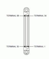
NI 5751 Pinout-Digital Connector
