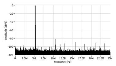
Figure 1. NI 5751 Characteristic Dynamic Performance, Spectrum – 64 k Samples, 5.3 MHz, -1 dBFS Input Signal
