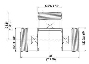
NOTE: T-adaptor is a non-matched 3 dB divider for low frequency applications. VSWR  $\geq$  2.0 when terminated 50  $\Omega$ .
