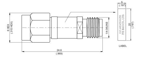
Nominal impedance:  $50\Omega+/-0.25\Omega$  over operating temperature range.
