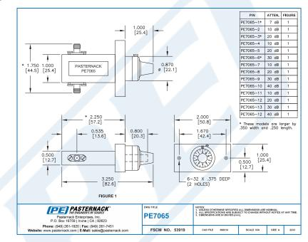
0 to 30 dB Rotary Continuously Variable Attenuator, SMA Female To SMA Female Rated To 5 Watts From 8 GHz To 12.4 GHz from Pasternack Enterprises has same day shipment for domestic and International orders. Our RF, microwave and millimeter wave products maintain a 99% availability and are part of the broadest selection in the industry.
