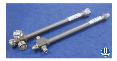
Microlab Model Dx-08 series of 2, 3 and 4 way Power Splitters has been designed to evenly split high power cellular and WiMAX signals with minimal reflections or loss. All joints are moisture sealed with o-rings to meet IP67. The mechanical shape allows easy attachment to wall using the supplied clips.
