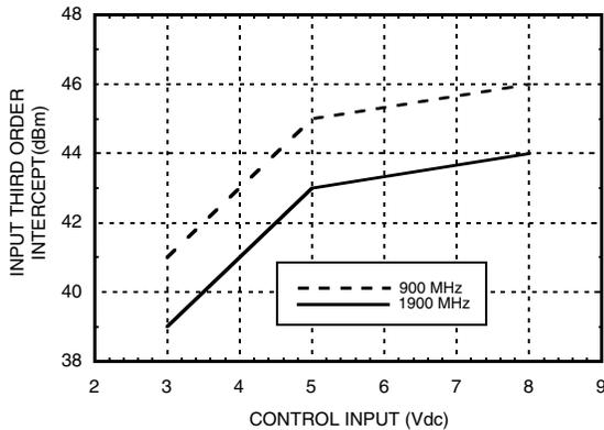
**Distortion vs. Control Voltage**
