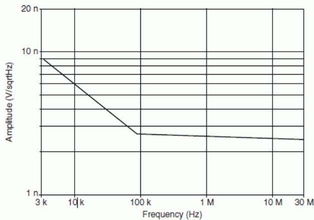
Representation of NI PCI-5105 Spectral Noise Density on 50 mV<sub>pk-pk</sub> Range, 50  $\Omega$  Input Impedance with Antialias Filter Enabled
