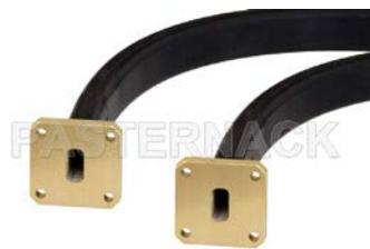
WR-51 Flexible Waveguide Twist With a Square Cover Flange Operating From 15 GHz to 22 GHz
