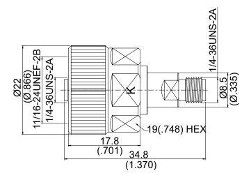
Note:Ruggedized K jack to be mounted directly on vector network analyzer.
