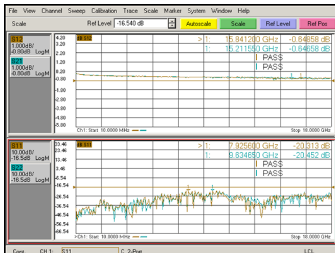
Test #1: SMA Male to SMA Male, 24 inches, DC -18 GHz
