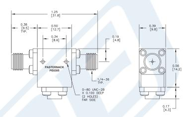
50 Ohm SMA Isolator Operating From 11 GHz to 18 GHz And 1 Watts With 20 dB Isolation from Pasternack Enterprises has same day shipment for domestic and International orders. Our RF, microwave and fiber optic products maintain a 99% availability and are part of the broadest selection in the industry.
