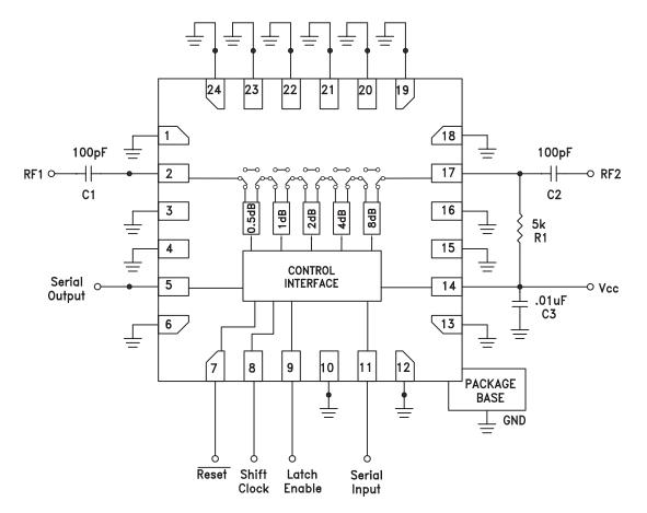
DC blocking capacitors C1 & C2 are required on RF1 & RF2. Choose C1 =  $C2 = 100 \sim 300 \text{ pF}$  to allow lowest customer specific frequency to pass with minimal loss. R1 = 5 kOhm is required to supply voltage to the circuit through either PIN 2 or PIN 17.
