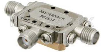
50 Ohm SMA Mixer Operating From 6 GHz to 18 GHz With an IF Range From 6 GHz to 18 GHz And LO Power of +10 dBm
