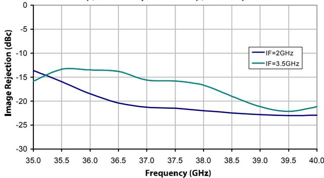
**XR1008-QB: LSB Image Rejection vs Frequency**
