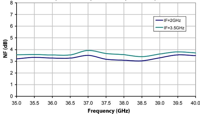
**XR1008-QB: LSB Noise Figure vs Frequency**
