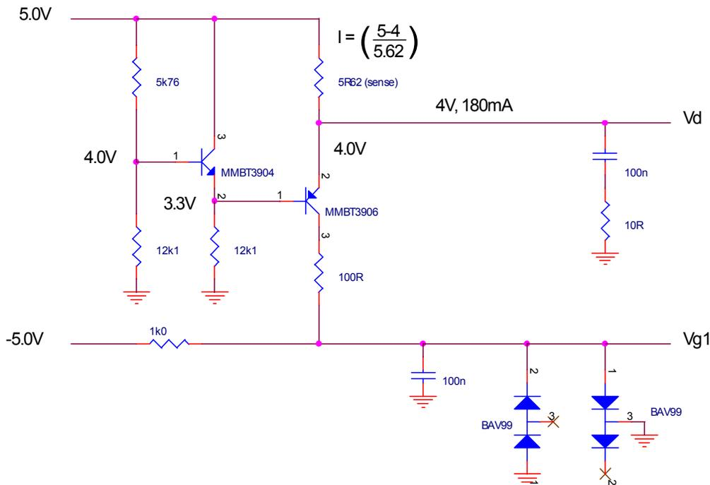
**App Note [3] USB/LSB Selection** - Please refer to the functional block diagram and pin-out table for biasing information. The device is operated by biasing  $V_D=4.0$  V with  $I_D=180$  mA by adjusting the applied voltage on VG1.
