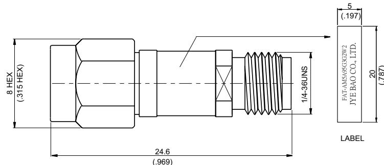
Nominal impedance:  $50\Omega \pm 0.25\Omega$  over operating temperature range.
