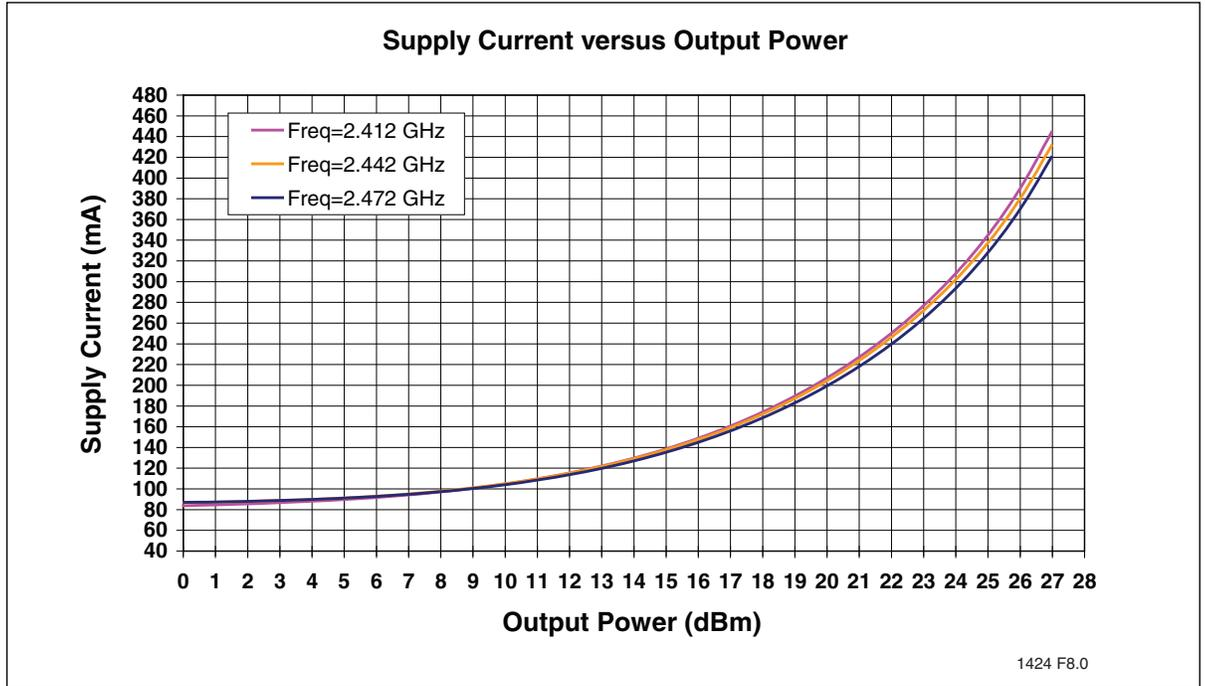
**Figure 21:**Total Current Consumption for 802.11g operation versus Output Power
