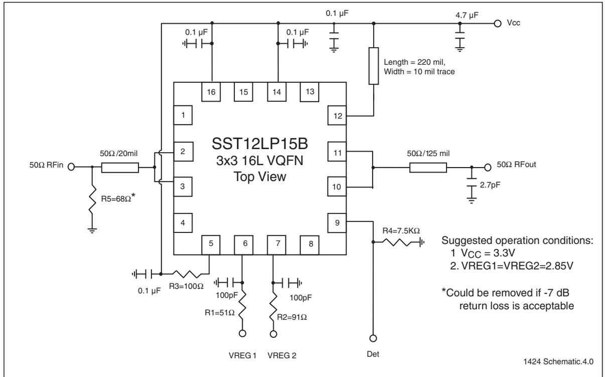
**Figure 10:** Typical Schematic for High-Linearity, 802.11b/g/n Applications for 16-contact VQFN, 3.3V
