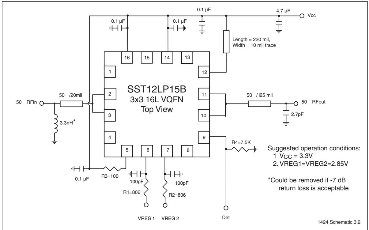
**Figure 23:** Typical Schematic for 3.3V, High-Efficiency 802.11b/g/n Applications for 16-contact VQFN
