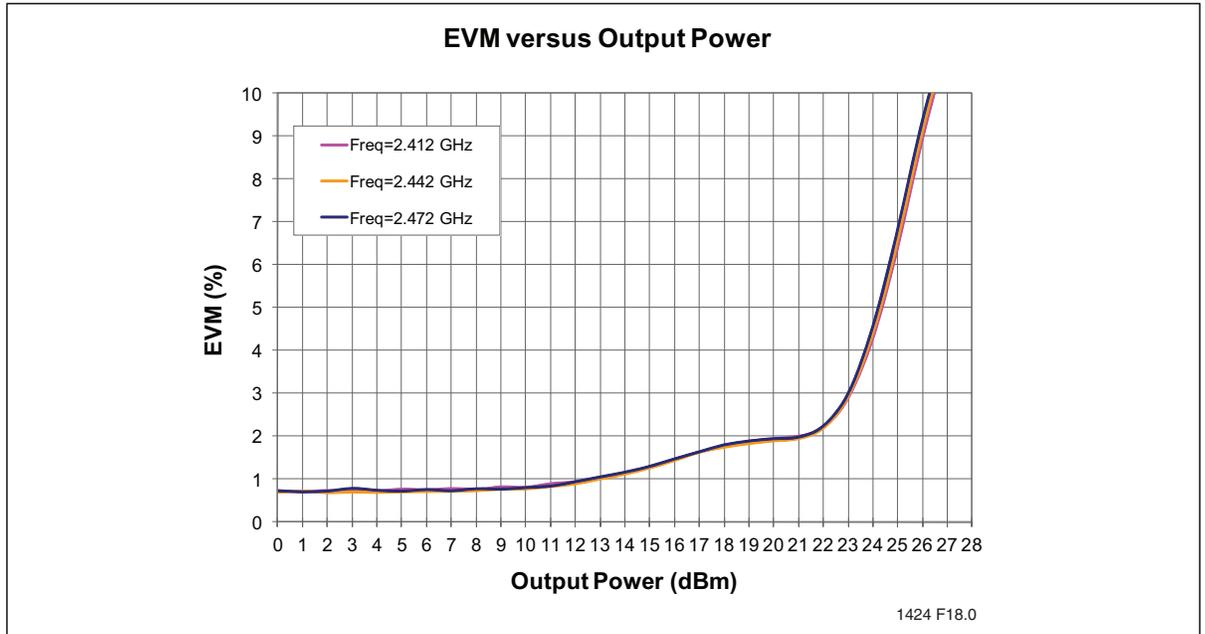
Figure 13: EVM versus Output Power measured with equalizer training set to sequence only
