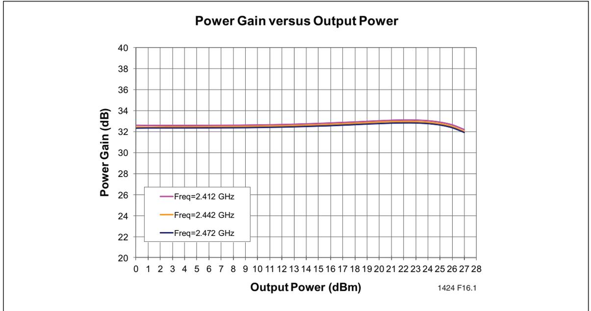
Figure 14: Gain versus Output Power
