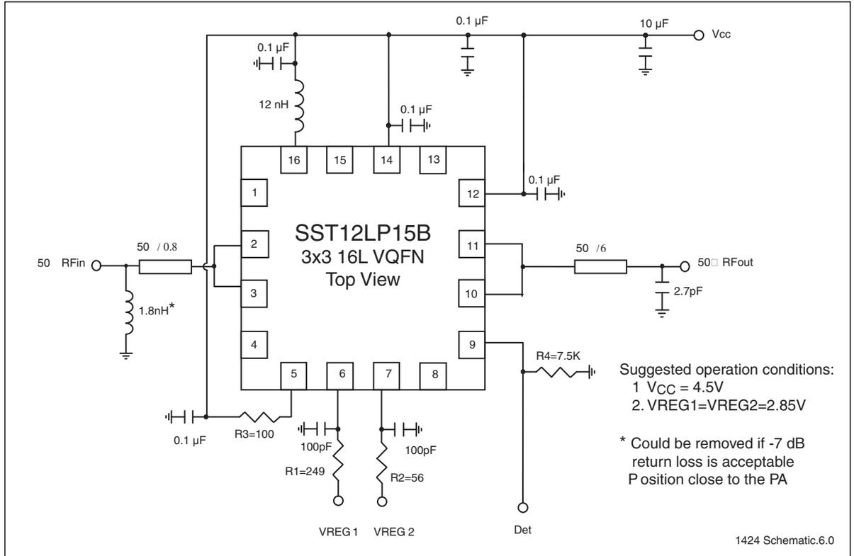
**Figure 24:** Typical Schematic for 4.5V, High-Efficiency 802.11b/g/n Applications for 16-contact VQFN
