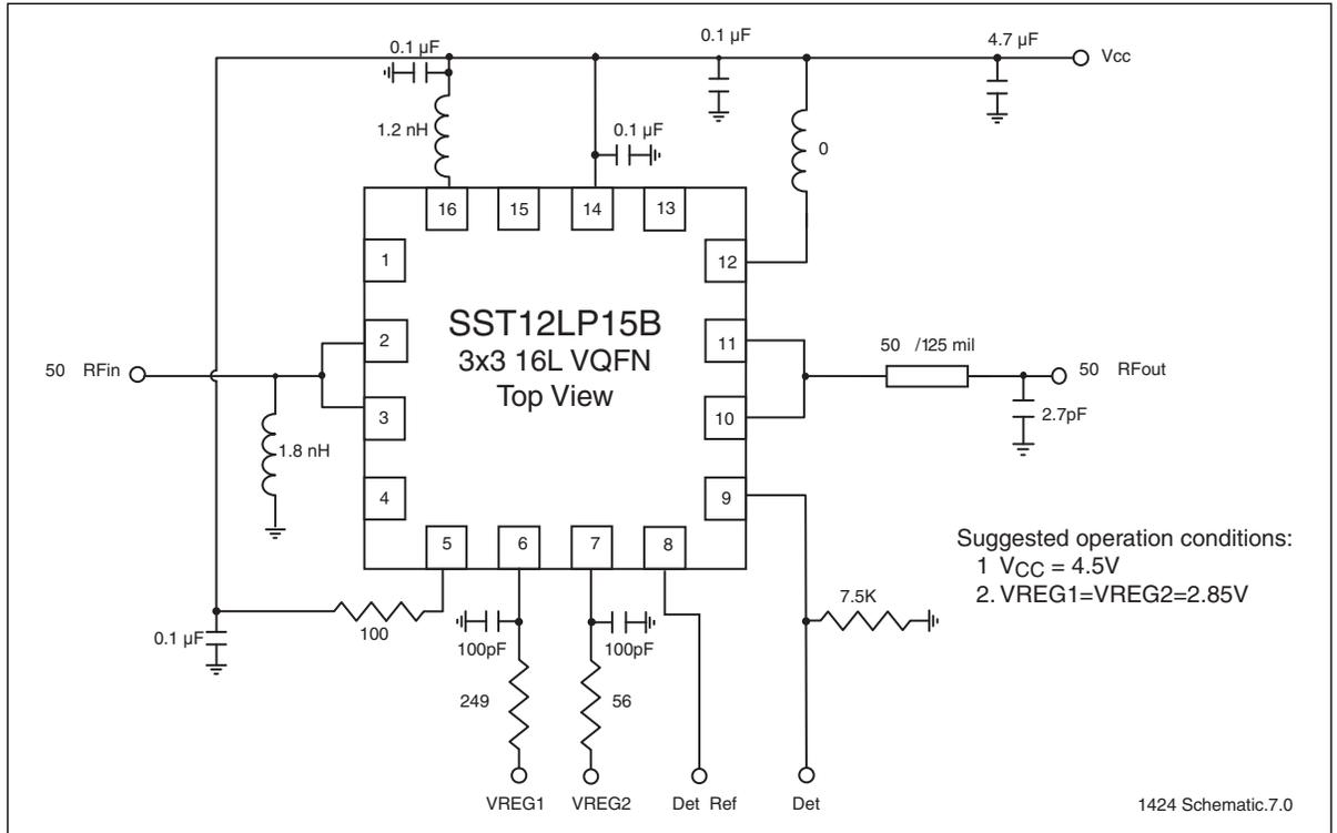
**Figure 11:** Typical Schematic for High-Linearity, 802.11b/g/n Applications for 16-contact VQFN, 4.5V
