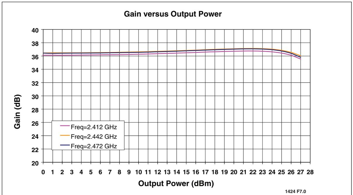
**Figure 20:** Gain versus Output Power
