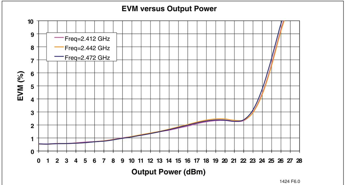
**Figure 19:** EVM versus Output Power measured with equalizer training set to sequence only
