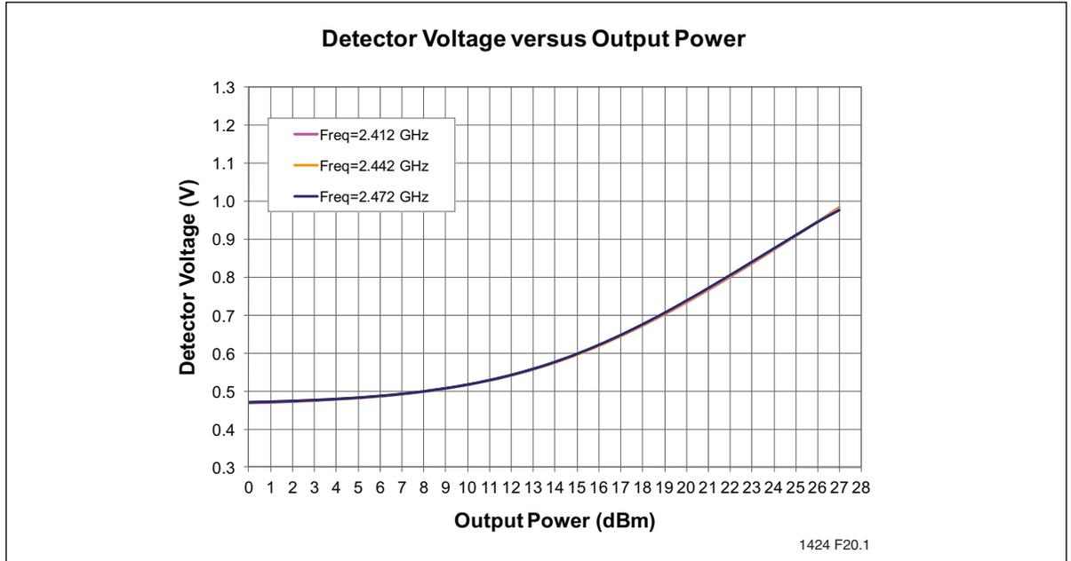
Figure 16: Detector Characteristics versus Output Power
