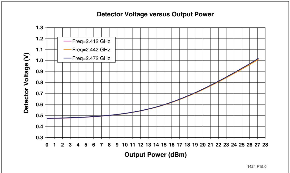
**Figure 9:** Detector Characteristics versus Output Power
