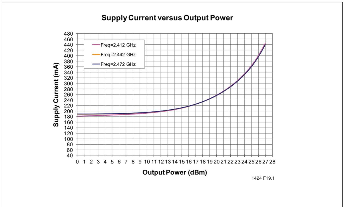
Figure 15: Total Current Consumption for 802.11g operation versus Output Power
