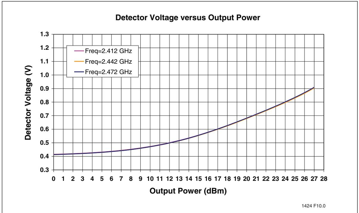
**Figure 22:**Detector Characteristics versus Output Power
