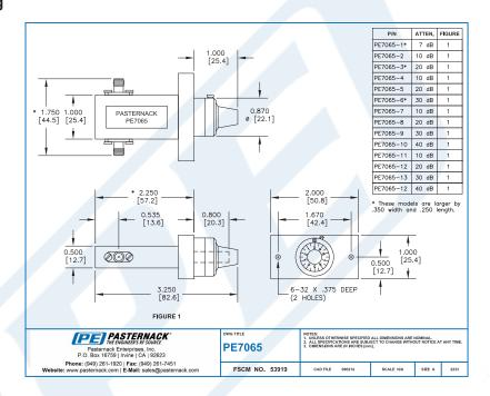
0 to 30 dB Rotary Continuously Variable Attenuator, SMA Female To SMA Female Rated To 5 Watts From 12.4 GHz To 18 GHz from Pasternack Enterprises has same day shipment for domestic and International orders. Our RF, microwave and millimeter wave products maintain a 99% availability and are part of the broadest selection in the industry.
