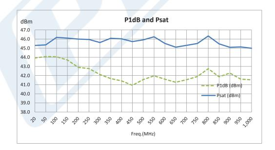
Click the following link (or enter part number in "SEARCH" on website) to obtain additional part information including price, inventory and certifications: 46 dB Gain, 25 Watt Psat, 20 MHz to 1,000 MHz, High Power High Gain Amplifier, 48 dBm IP3, SMA PE15A5031
