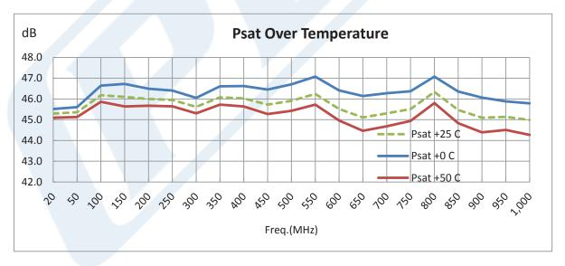
Click the following link (or enter part number in "SEARCH" on website) to obtain additional part information including price, inventory and certifications: 46 dB Gain, 25 Watt Psat, 20 MHz to 1,000 MHz, High Power High Gain Amplifier, 48 dBm IP3, SMA PE15A5031
