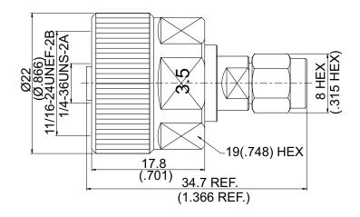
Note:Ruggedized 3.5 jack to be mounted directly on vector network analyzer.
