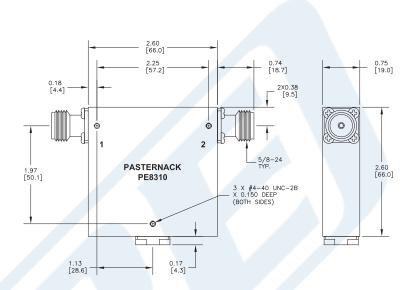
50 Ohm N Isolator Operating From 1 GHz to 2 GHz And 10 Watts With 18 dB Isolation from Pasternack Enterprises has same day shipment for domestic and International orders. Our RF, microwave and fiber optic products maintain a 99% availability and are part of the broadest selection in the industry.
