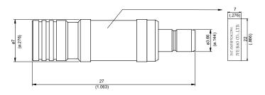
Nominal impedance:  $50\Omega$ +/-0.25 $\Omega$  over operating temperature range. Operating temperature range: -50 degrees Celcius to +80 degrees Celcius.
