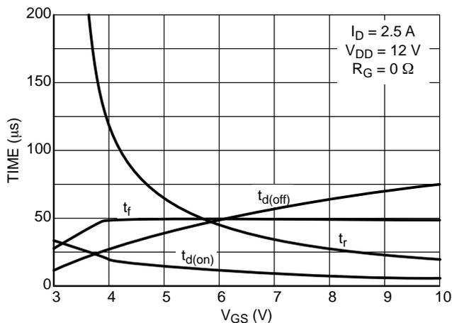
Figure 16. Resistive Load Switching Time vs. Gate-Source Voltage
