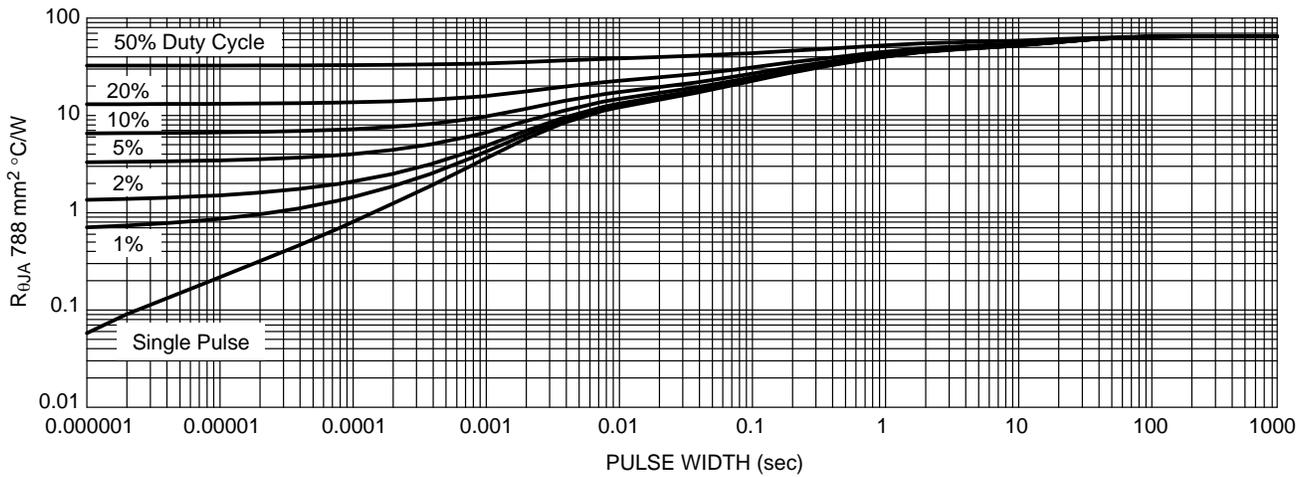
Figure 21. Transient Thermal Resistance – DFN Package
