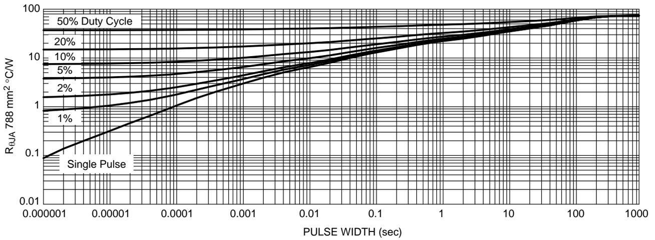
Figure 20. Transient Thermal Resistance – SOT-223 Package
