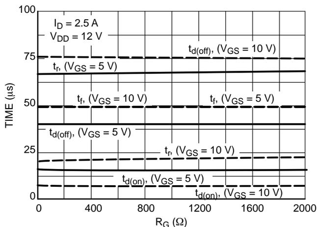
Figure 18. Resistive Load Switching Time vs. Gate Resistance
