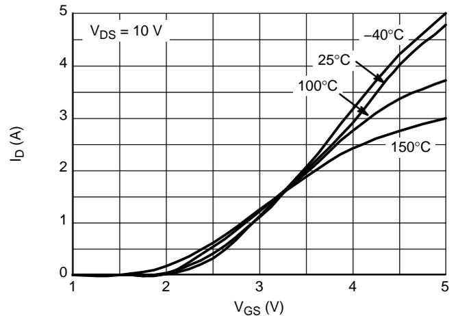
Figure 7. Transfer Characteristics
