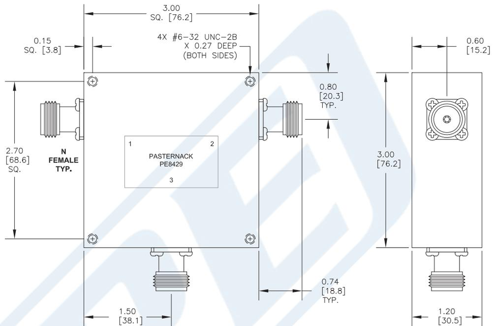
50 Ohm N Circulator Operating From 330 MHz to 403 MHz And 150 Watts With 20 dB Isolation from Pasternack Enterprises has same day shipment for domestic and International orders. Our RF, microwave and millimeter wave products maintain a 99% availability and are part of the broadest selection in the industry.
