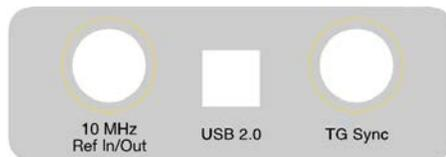
1. 10 MHz Reference input / output. Used in the legacy software in some modes.
