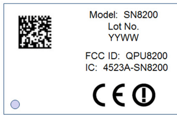
FIGURE 7.2 Typical SN820X/820XUFL module marking
