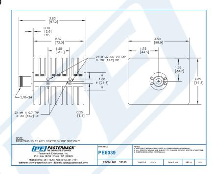
Medium Power 50 Watts RF Load Up To 18 GHz With N Female Input Square Body Black Anodized Aluminum Heatsink from Pasternack Enterprises has same day shipment for domestic and International orders. Our RF, microwave and millimeter wave products maintain a 99% availability and are part of the broadest selection in the industry.
